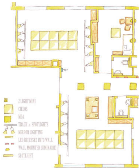
Fig. 4-1. Preliminary design sketch of common area with both luminous ceilings (bottom right – eat-in kitchen; bottom left – living room)
