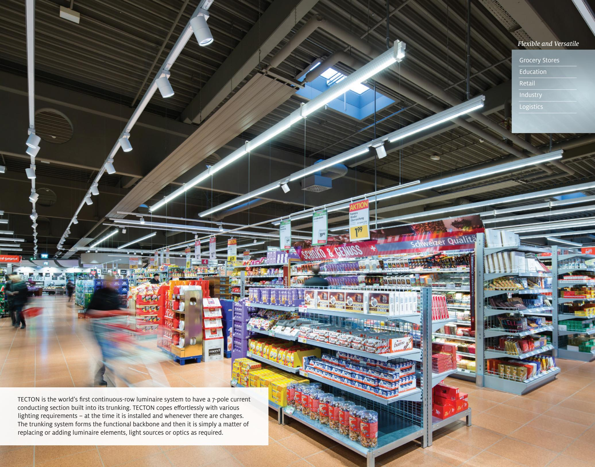
TECTON is the world's first continuous-row luminaire system to have a 7-pole current conducting section built into its trunking. TECTON copes effortlessly with various lighting requirements – at the time it is installed and whenever there are changes. The trunking system forms the functional backbone and then it is simply a matter of replacing or adding luminaire elements, light sources or optics as required.
