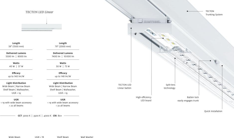
Long continuous rows with one electrical feed - up to 195 ft. max. run (120 V) | 449 ft. max. run (277 V)\*
