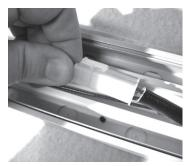
Reattach the wireway cover with the screws you removed in Step 6.
