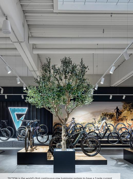
TECTON is the world's first continuous-row luminaire system to have a 7-pole current conducting section built into its trunking. TECTON copes effortlessly with various lighting requirements – at the time it is installed and whenever there are changes. The trunking system forms the functional backbone and then it is simply a matter of replacing or adding luminaire elements, light sources or optics as required.
